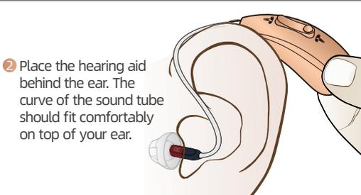
2 Place the hearing aid behind the ear. The curve of the sound tube should fit comfortably on top of your ear.
