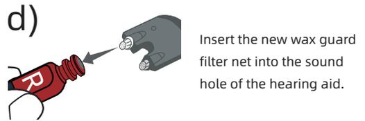
Insert the new wax guard filter net into the sound hole of the hearing aid.
