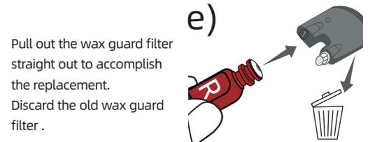
Pull out the wax guard filter straight out to accomplish the replacement. Discard the old wax guard filter.
