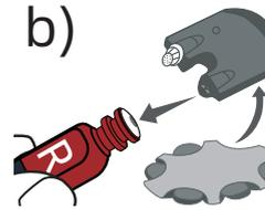
Align the removed end of the wax guard filter with the sound hole of the hearing aid and insert.
