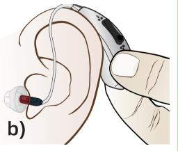
3. Put the stabilizer bar into the outer bowl of the ear. It can be trimmed according to the size of your ears.
