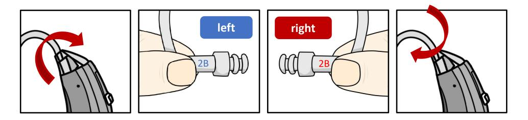
**1.** Remove the sound guide by rotating the bottom of the sound tube counterclockwise.
